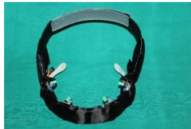
Figure 1: Neck Strap with IR sensors
