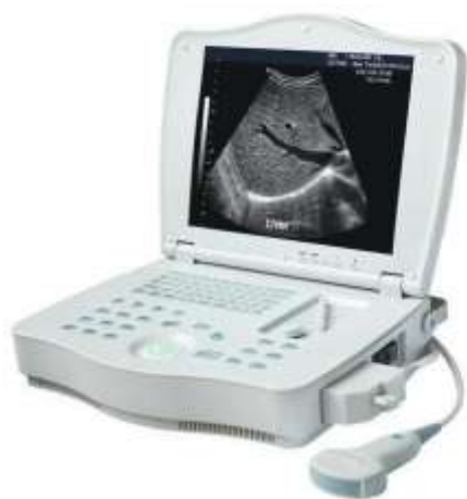
Figure 1 :An ultrasound scanner is a medical device that uses high-frequency sound waves to produce real-time images of internal body structures.
