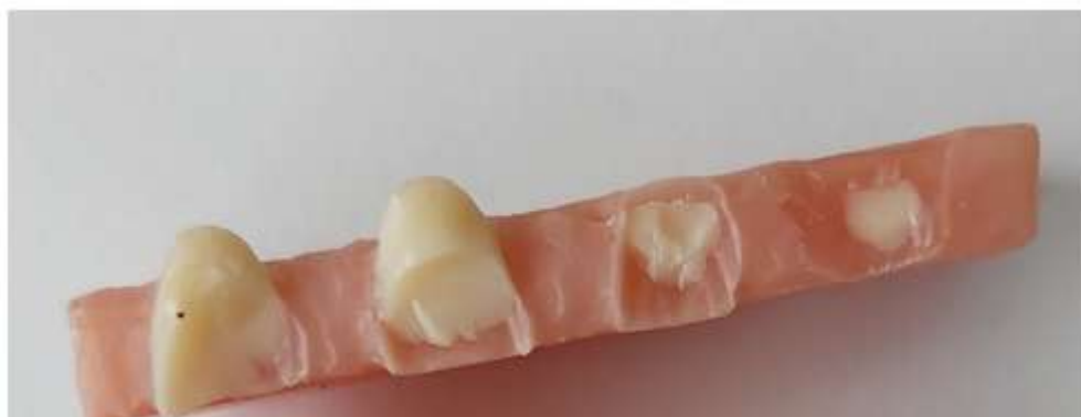
Figure 4 Cohesive type of adhesin between acrylic teeth and plate
