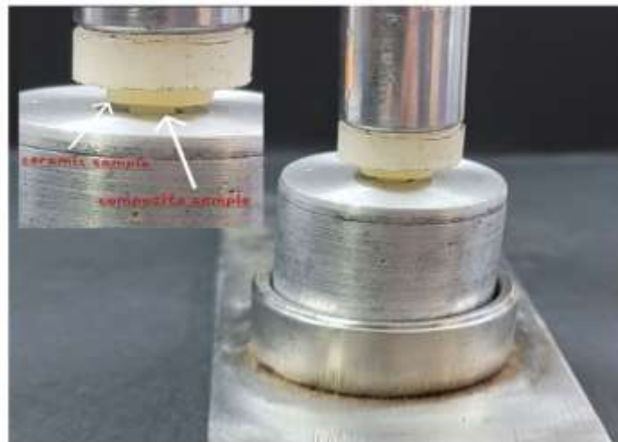
Fig.2 Special designed device for cementation
