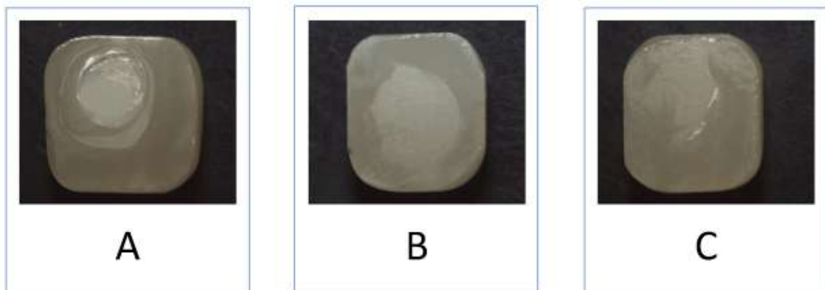
Fig.6 Failure patterns: A; cohesive failure within composite resin disk with remaining resin cement. B; Adhesive failure between vita block and resin cement. C; mixed failure illustrated the remaining resin cement and composite resin disk.
