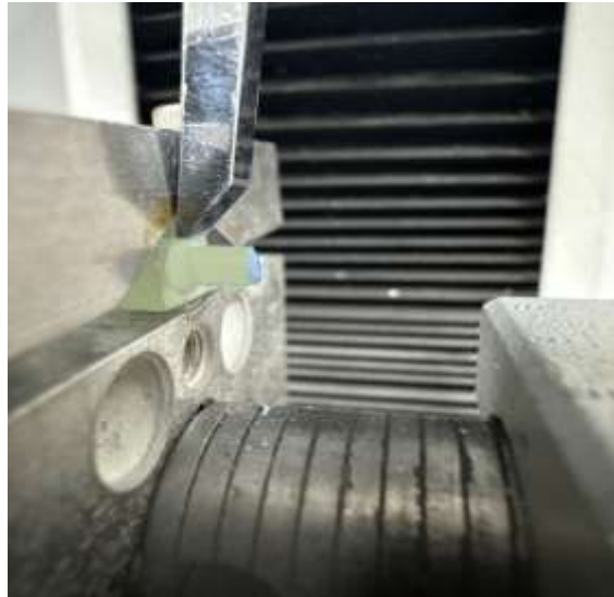
Fig.3 Application of the load for shear test
