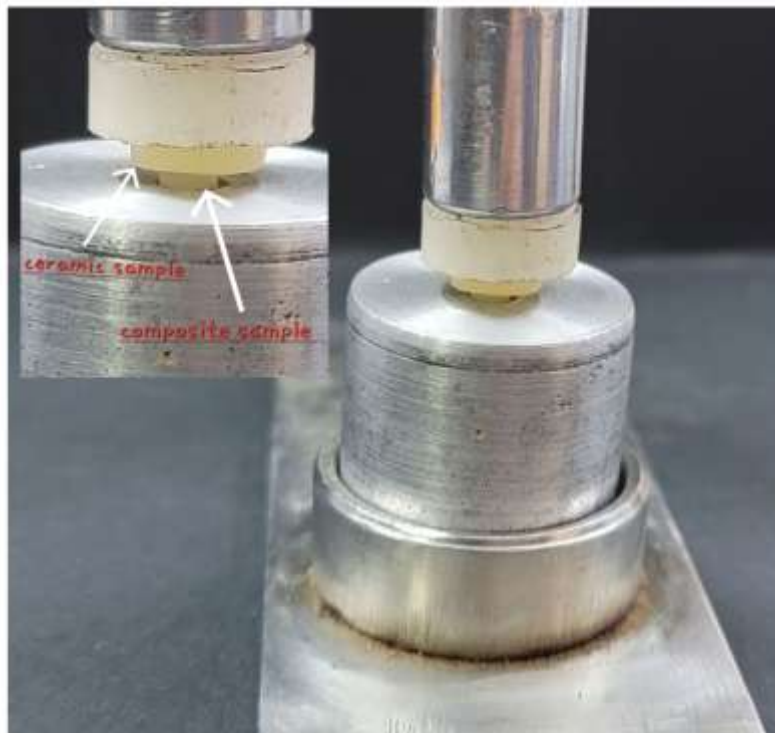
Fig.2 Special designed device for cementation
