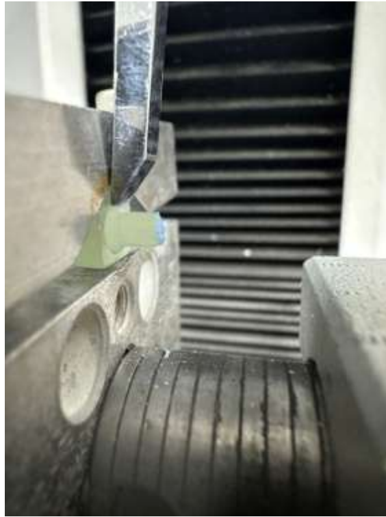
Fig.3 Application of the load for shear test
