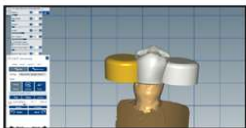
Figure 1: Adding a special extension to restoration with dimensions 6 \times 4.5 \times 5 mm.
