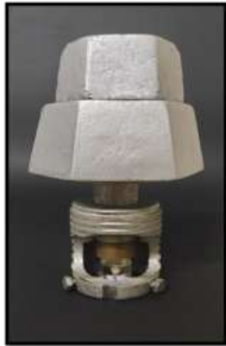
Figure 4: Endo-crown restoration under constant load in a special loading device.
