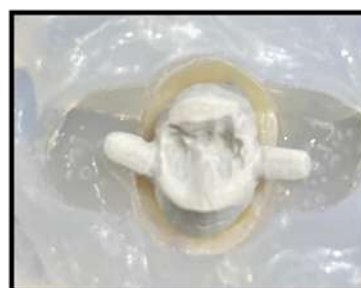
Figure 3: PEEK core within silicon mold.
