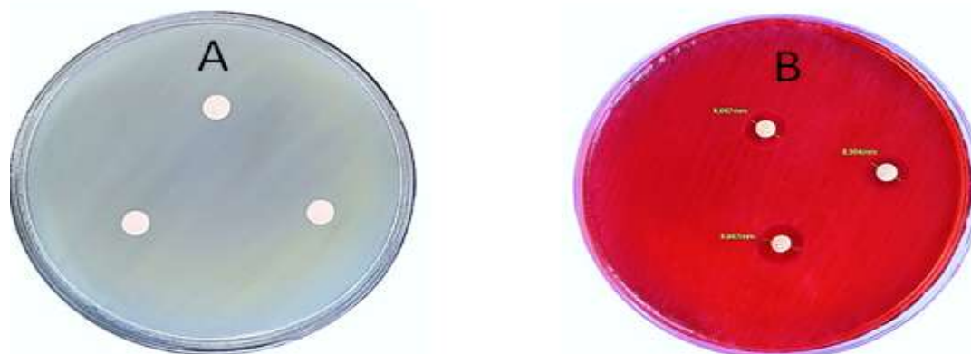
Figure 6: Antibacterial activity of Group3 (composite modified with CuO 0.01%) against A) E. coli, B) S. mutans.
