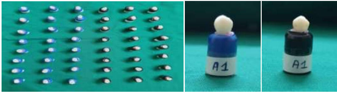
Figure 1: Premolar samples mounted in acrylic blocks and labelled
