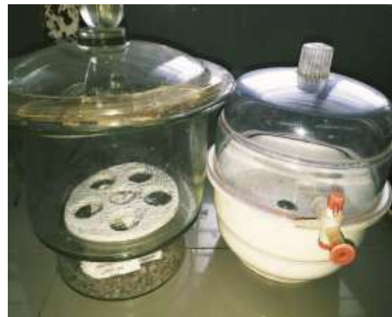
(Desiccator unit used in the study for removing excess moisture from study samples)
