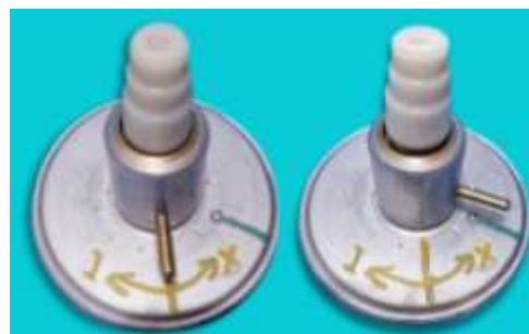
Figure 2: mold made of copper and Teflon with a regulator.
