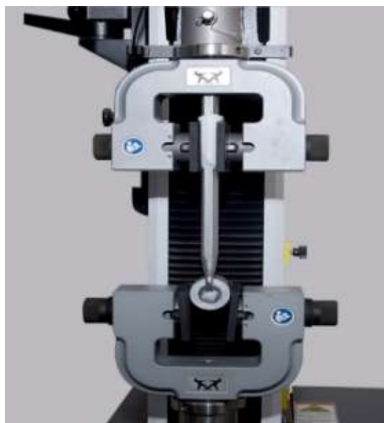
Figure 3: Instron universal testing machine with zirconia block infrastructure veneered with e.maxceram mounted inside.
