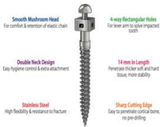
Figure 2- Specifications of extra-alveolar bone screw
