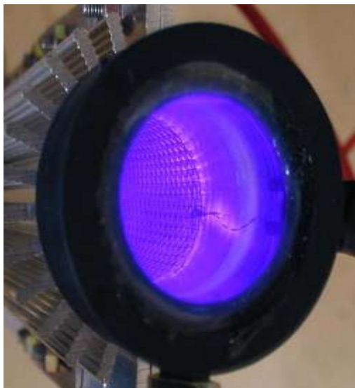
Fig.3:Corona discharge ozone generator
