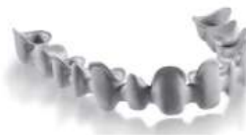
Fig 6: A 14-unit bridge manufactured in the SLM process made from the alloy Wirobond C+
