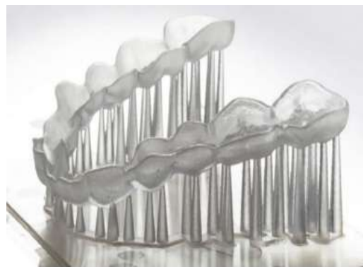
Fig. 3: Splint immediately after the 3D printing process with the printing base and support structure. The CAD design is done using ‘Splint designer’. The implementation was performed in the CAM process using stereolithography.
