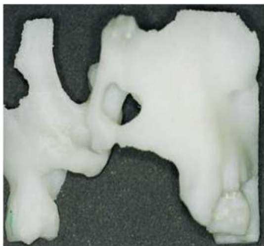
Fig. 1: The first patient treated by Dawood A 11 with the help of 3D printing in 1999 Frontal view of the 3D printed medical model, printed with Fused Deposition Modelling (FDM) technology, which
