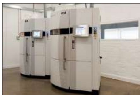
Fig 7: Selective laser Sintering 3D printer
