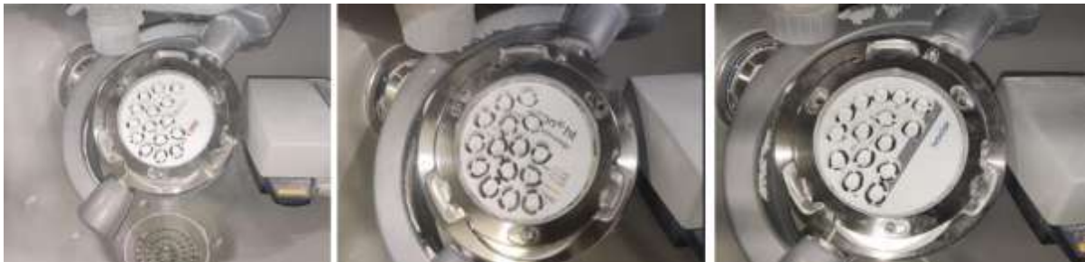
FIGURE5: Crowns milled through respective discs
