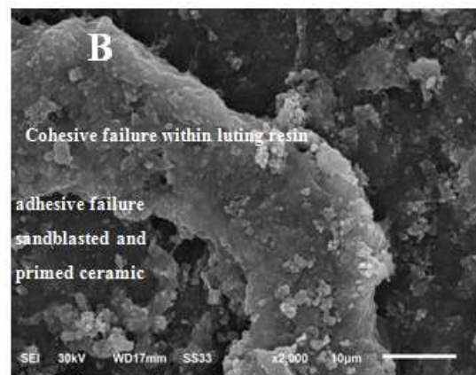
Fig. (1) Representative SEM micrograph from group GSP, (A) and group CSP, (B) demonstrating mixed failure pattern between hybrid ceramic and luting cement.
