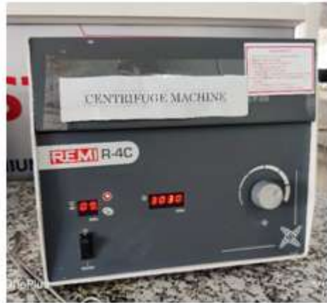
FIGURE 16: Collected blood is centrifuged in a centrifugation machine at 3000rpm for 10 minutes
