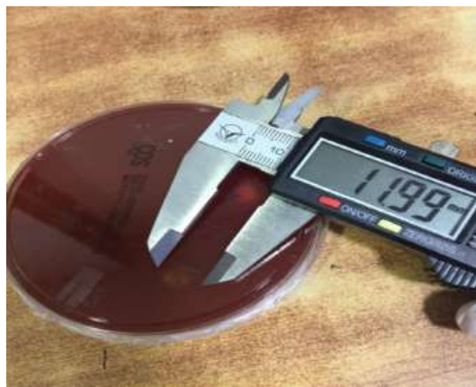
Fig. 5 MEASUREMENT OF ZONES OF INHIBITION BY DIGITAL VERNIER CALIPER
