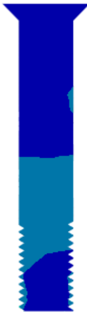
Figure 3D showing stresses in abutments crew
