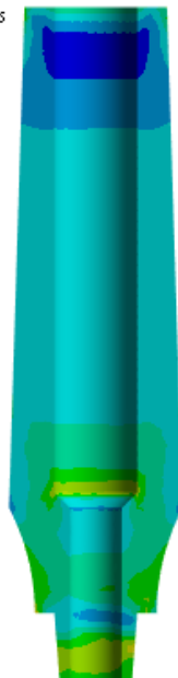
Figure 5C showing stresses in abutment
