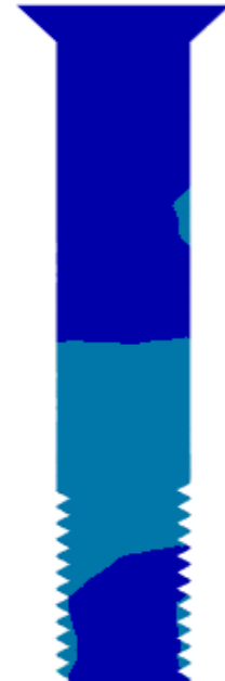
Figure 4D showing stresses in abutments crew
