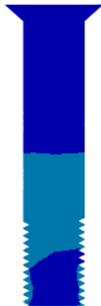
Figure 1D showing stresses in abutments crew
