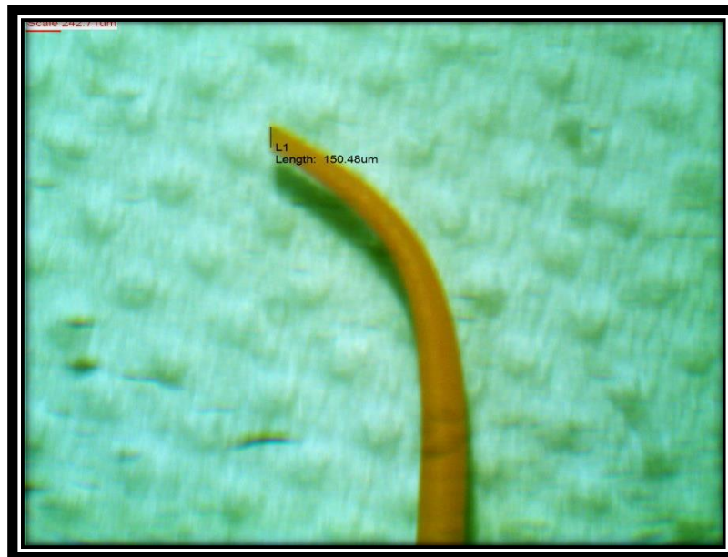
Image 2: Representative stereomicroscopic image of apical tip diameter for WaveOne group
