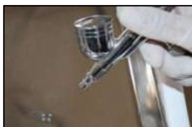
Figure 3 PHOTODYNAMIC SPARY COATED USING AIRBRUSH
