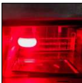
Figure 4 EXPERIMENT SAMPLES EXPOSED TO RED LED LIGHT FOR PHOTOACTIVATION
