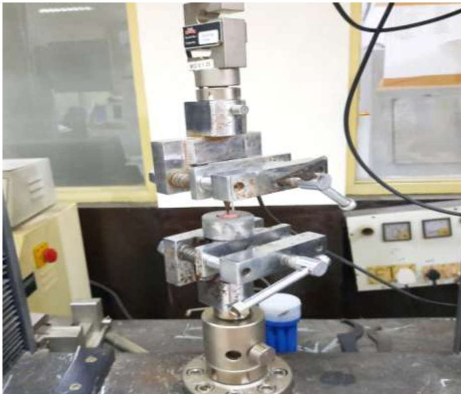
FIGURE 3: INSTRON TESTING MACHINE USED FOR TESTING THE SAMPLES
