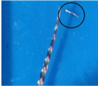
Figure 5: Broken File fragment[3mm]
