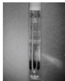
Fig 8 : Side firing fiber. At the top of the fiber the beam is diverted in a 90^\circ angle.
