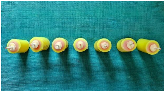
FIGURE 4. Specimens mounted with autopolymerizing resin in a PVC pipe.
