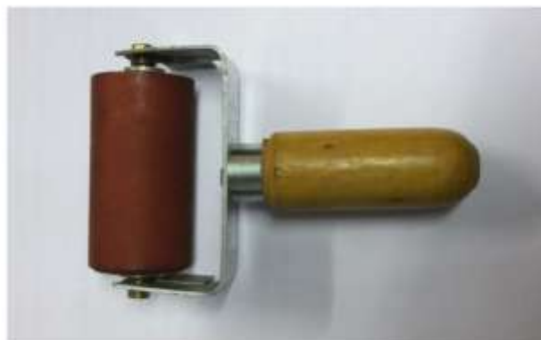
Figure 1. Roller used for spreading ink.
